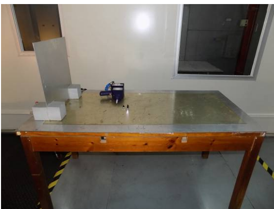
7.3. Photo of electrostatic discharge Immunity measurement (E.S.D.)
